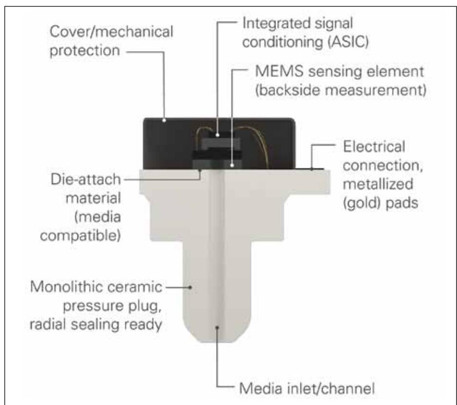
▲ Fig. 1: Monolithic Metallized Plug Cross Section.
