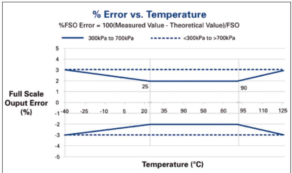
▲ Fig. 3: Output Signal Error vs. Temperature.
